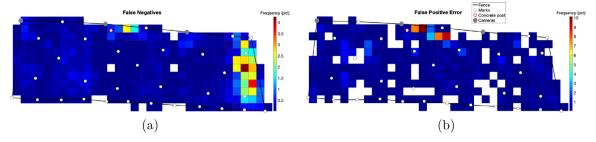
**Fig. 3.** Spatial distribution of the detection error for data set  $D_1$ . Spatial distribution of the false negative detections (a) and false positive detections (b). The red areas in (a) are the areas where the detection errors are concentrated. 46% of the false positive errors and 53% of the false negative errors are inside the red areas. (For interpretation of the references to colour in this figure legend, the reader is referred to the web version of this article.)
