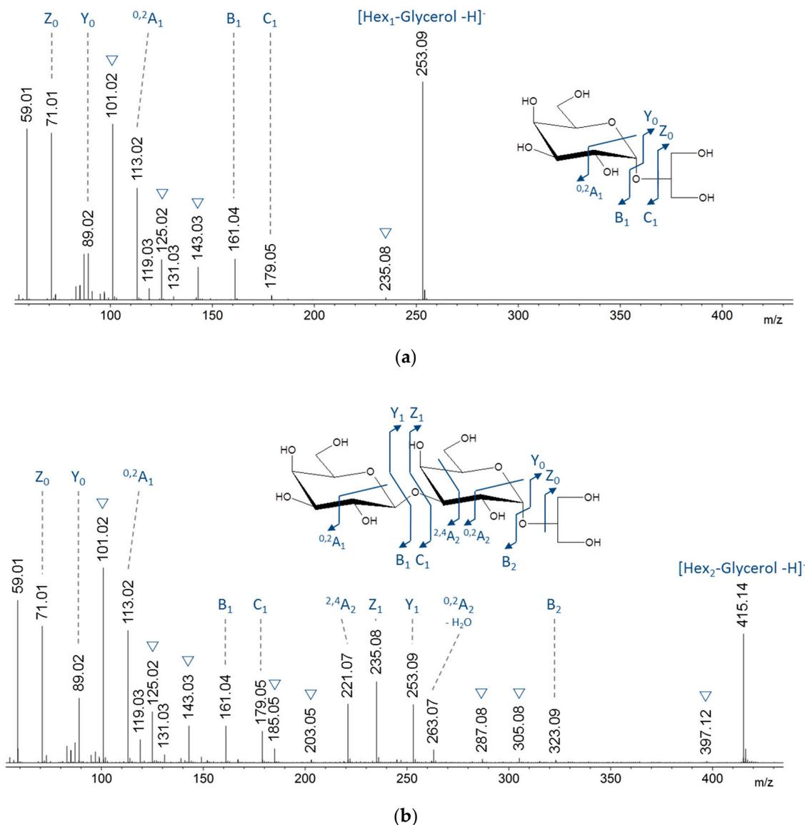
**Figure 3.** ESI-MS/MS (–) spectra of the hexose-glycerol (a) and the (hexose)<sub>2</sub>-glycerol (b) observed at  $m/z$  253.09 and  $m/z$  415.14, respectively. ▽: Water losses.
