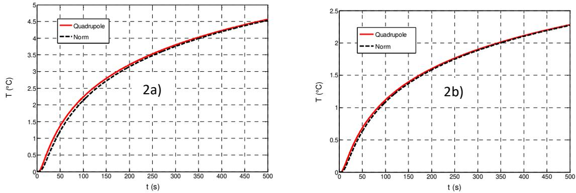
Figure 2: Temperature of the thermocouple simulated with the model of the standard and with the quadrupolar model: 2a)  $\lambda_s = 0.1 \text{ W m}^{-1} \text{K}^{-1}$  ; 2b)  $\lambda_s = 0.2 \text{ W m}^{-1} \text{K}^{-1}$
