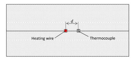
Figure 1: Schematic diagram of the parallel hot wire method
