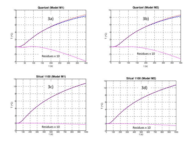
Figure 3: COMSOL simulations (--), quadrupolar model (--) and residues×10 for two materials
