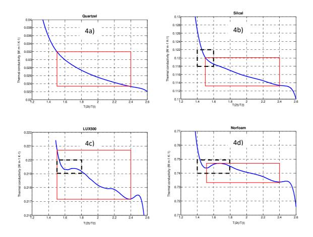
Figure 4: Thermal conductivity of the four materials estimated with the method of the standard ISO 8894-2 with sample dimensions  $200 \times 100 \times 50 \text{ mm}^3$  and d = 15 mm.
