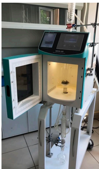
Figure 5. Reactor for solvent-free microwave-assisted extraction.
