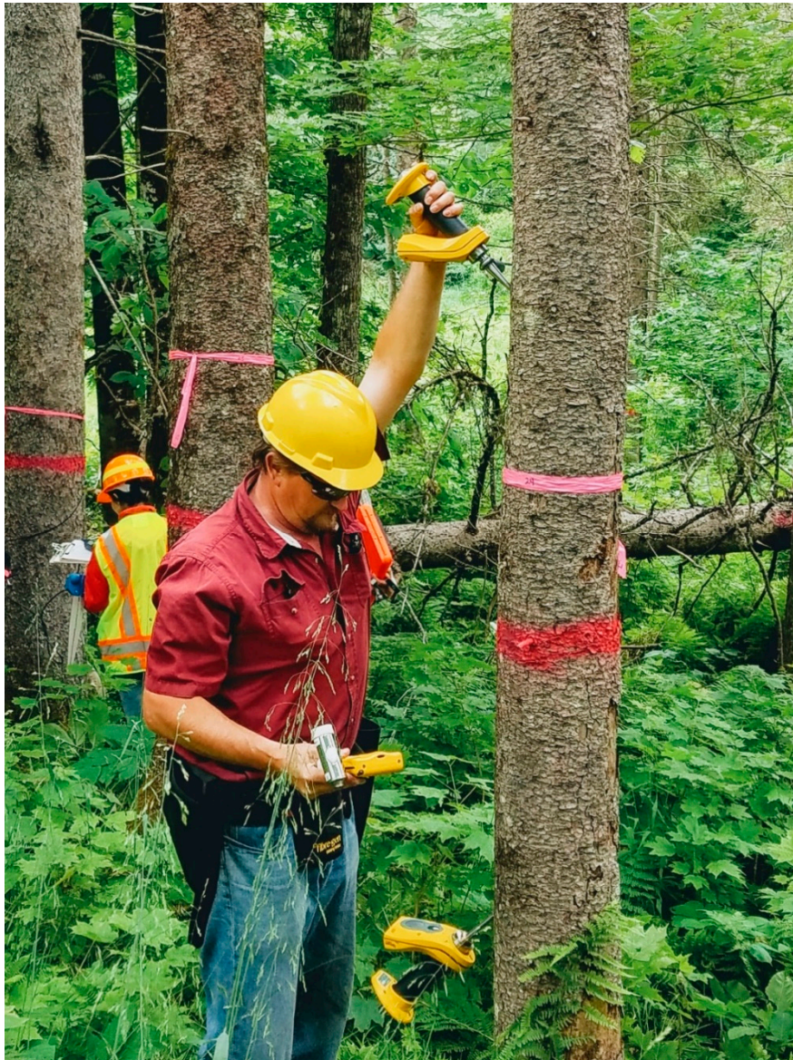
Figure 2. A portable time of flight (TOF) acoustic tool for measuring acoustic velocity (AV) in standing trees (photo credit: Xiping Wang).
