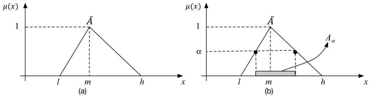
Figure 2. (a) TFN  $\tilde{A}$ ; (b)  $\alpha$ -cut of a TFN,  $A_\alpha$
