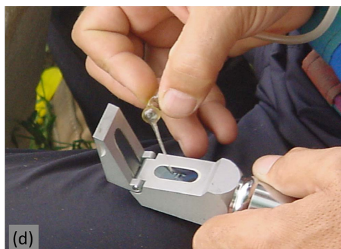
Fig. 2. Illustration of the nectar collection with the capillary pipet of the ICDA: general view of the device (a), nectar aspiration on Helianthus annuus and Lamium purpureum (b), field balance (c), refractometer (d)
