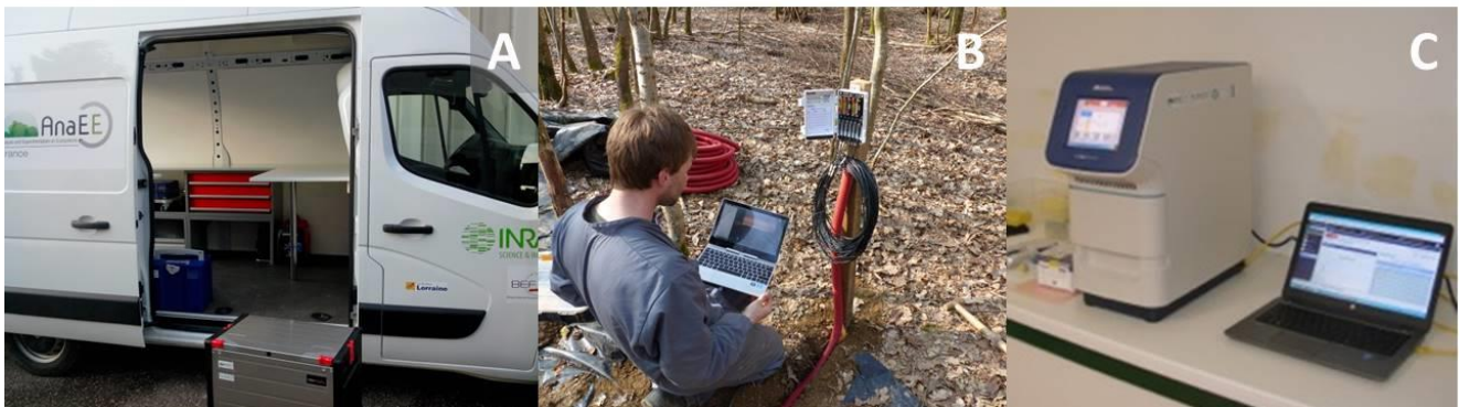
Fig. 8. The Mobile Platform for Observation and Experimentation in Terrestrial Ecosystems (E). a- View of the truck. b- Monitoring of soil water content using decagon probes. c- qPCR device
