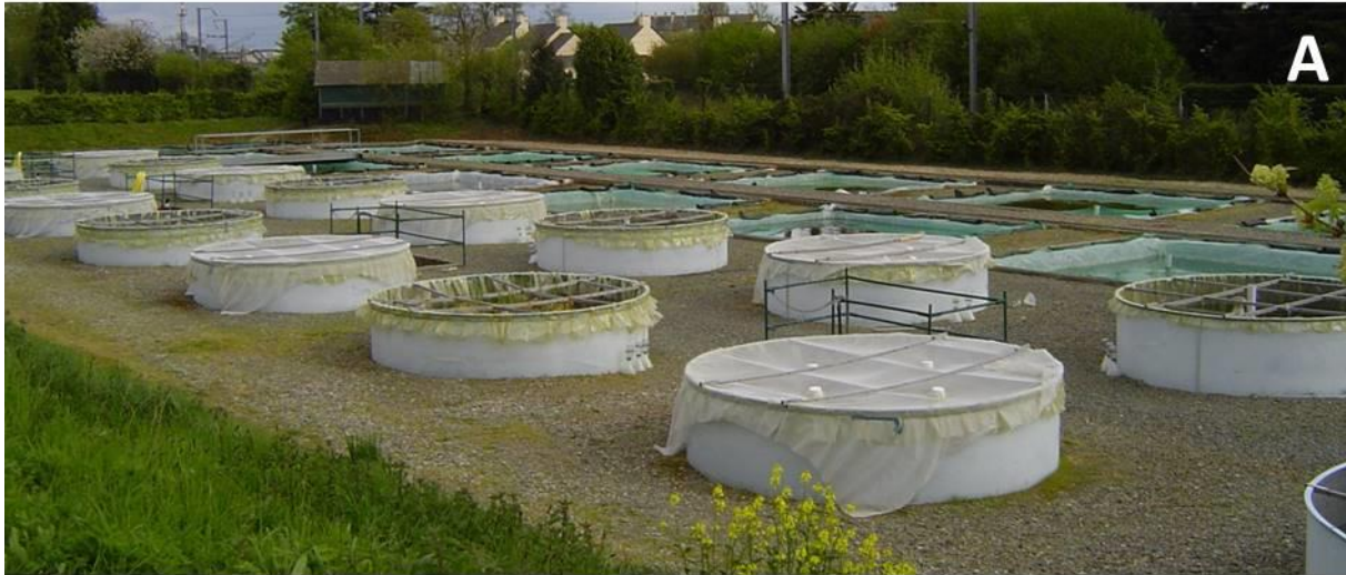
Fig. 5. Examples of PEARL experimental facilities. a. Mesocosm platform. In the foreground, the series of 16 circular mesocosms (volume: 9 m 3 ), at the back, 12 rectangular mesocosms (volume 30 m 3 ). Schematic representation of a mesocosm with some sampling systems. b. –Schematic view of a pond mesocosm (modified from Caquet et al. 2001. EIS emerging insect sampler, Mac macrophytes, MdIS macrophyte-dwelling Invertebrate Sampler, PS Periphyton-Sampler, SdIS sediment- dwelling Invertebrate Sampler, Sed Sediment)
