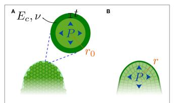
FIGURE 2 | Two mechanical models for the shoot apical meristem. (A) A homogeneous cellular aggregate. (B) A shell under pressure (negligible internal walls)
