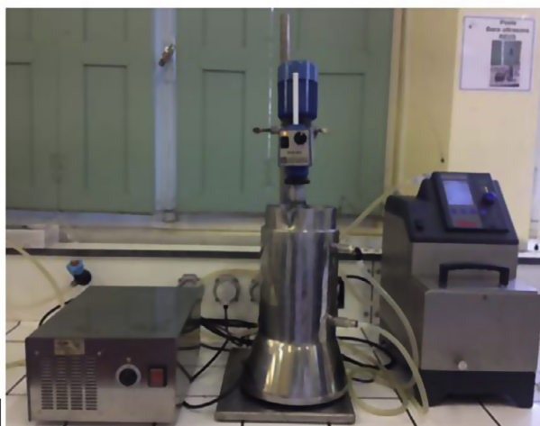
Fig. 1. Laboratory ultrasonic device (3L) used for ultrasound-assisted extraction by maceration (UAM).
