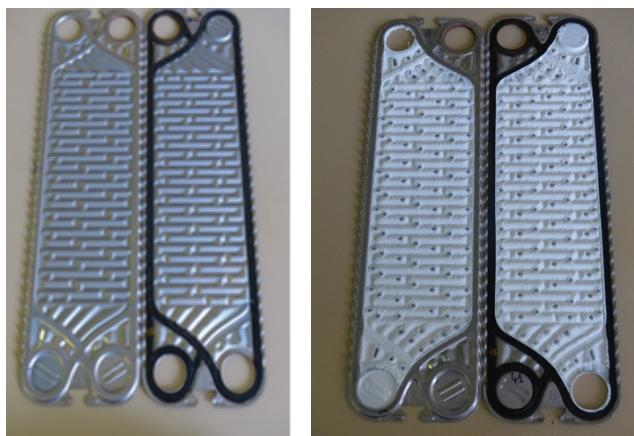
FIGURE 6: Pictures of the deposit collected on heat exchanger surface in the first and last channels of the PHE.
