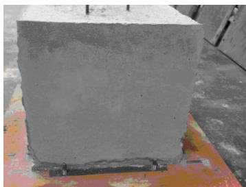
241 Fig. 7: Facing obtained with vegetable oil
