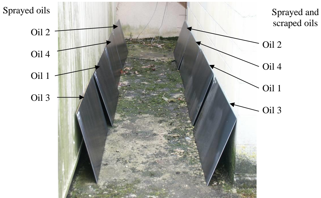
Fig. 11: Formwork surface storage zone
