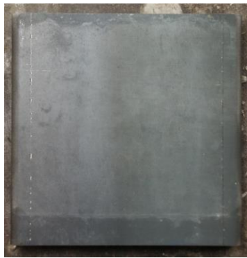
85 86 87 88 89 90 Fig. 2: New formwork surface
