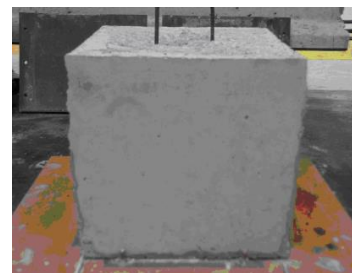
Fig. 8: Facing obtained with mineral oil
