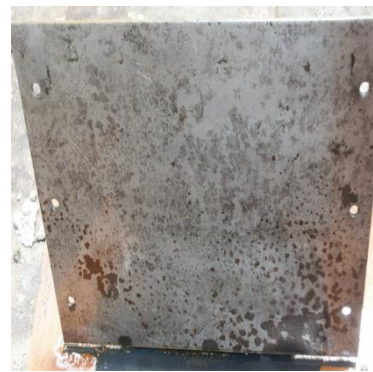
Fig. 3: Used formwork surface
