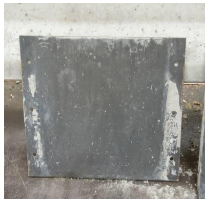
Fig. 10: Formwork obtained with mineral oil
