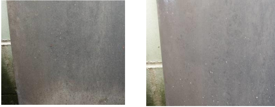
Fig. 14: Micrographs both before and after storage of sprayed oil 2
