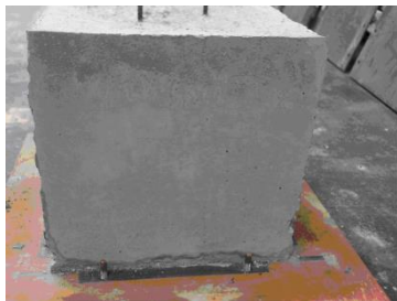
Fig. 7: Facing obtained with vegetable oil
