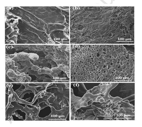
**Fig 3.** Scanning electron micrographs showing the surface morphologies of covalently cross-linked MBAX-4 (a,c,e) and MBAX-6 (b,d,f) gels: (a-b) without degradation and after; (c-d) 18 and (e-f) 36 hours of incubation with a mixture of *Bifidobacterium* strains (*B. longum*, *B. adolescentis*). All samples are at 350x magnification.
