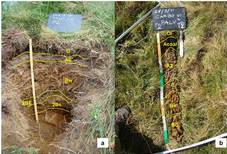
Figure 1. Soil profile at the control site (Panel a) and the charcoal hearth (Panel b). The letters indicate different pedologic horizons. In the charcoal hearth the dark anthropogenic layer (Acoal; 0–10 cm) can be easily identified. doi:10.1371/journal.pone.0091114.g001
