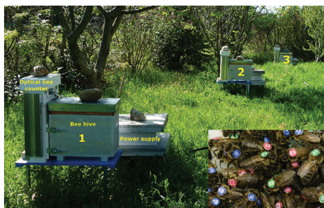
Fig. 2. Optic bee counters in the field measuring the activity of honey bees with coloured tag numbers. The optic bee counter (at the entrance of the hive) and the power supply (next to the hive) were protected from climatic events by a wood box covered with a metal top. Bees identified with coloured tag numbers are shown in the inset.
