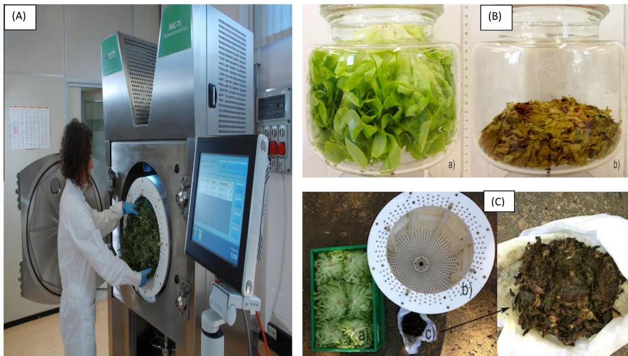
Fig. 1. (A) Pilot scale microwave hydrodiffusion and gravity apparatus. (B) Volumetric reduction of salad through water exhaustion by microwave hydrodiffusion and gravity technique: (a) fresh salad, (b) dry salad after microwave process. (C) Volumetric reduction of salad batch through water exhaustion by microwave hydrodiffusion and gravity technique, pilot reactor, (a) fresh salad batch, (b) reactor, (c) biomass after MHG reduction.
