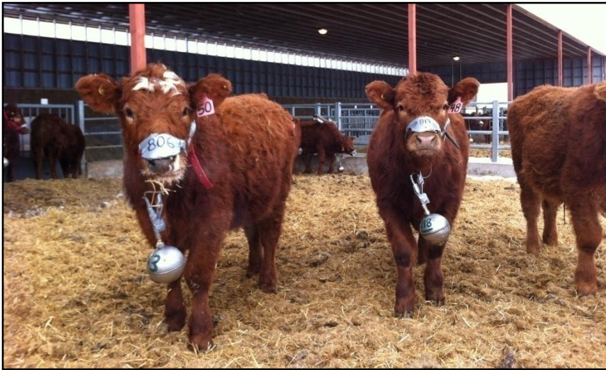
Figure 2. Cattle wearing the methane collection devices
