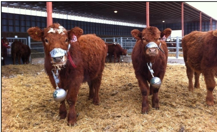
Figure 2. Cattle wearing the methane collection devices
