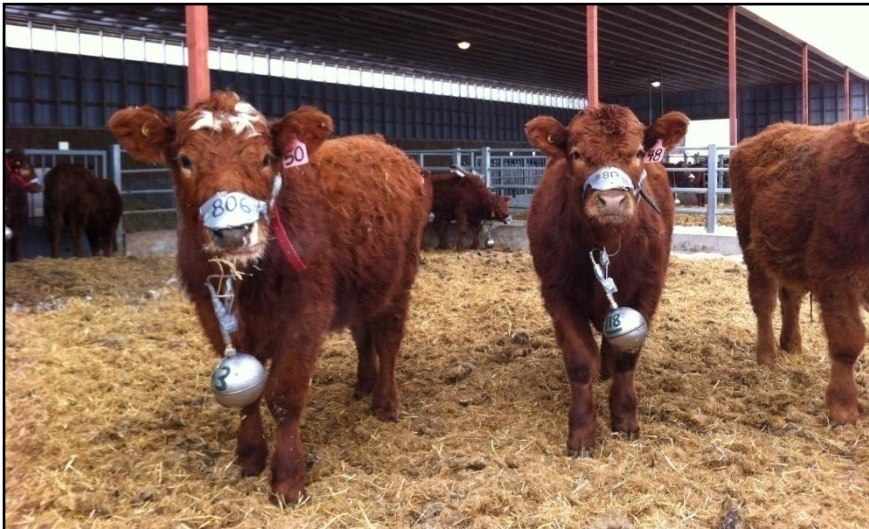
Figure 2. Cattle wearing the methane collection devices
