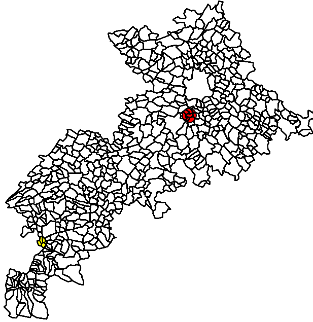
Figure 5: Municipalities composing Haute-Garonne. The red area corresponds to the impacted area when located at an arbitrary municipality for a radius of 3 km. The yellow area corresponds to the impacted area at the optimal location for the same radius.
