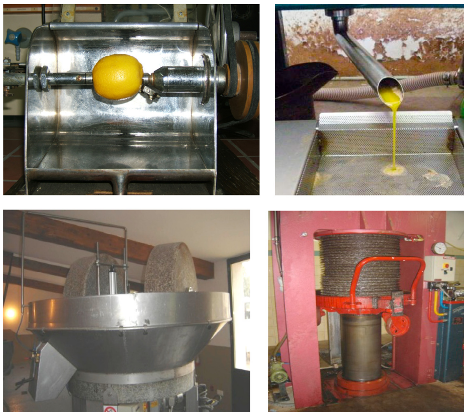
Fig. 2. Conventional techniques of solvent-free extraction for olive oil and citrus essential oil.
