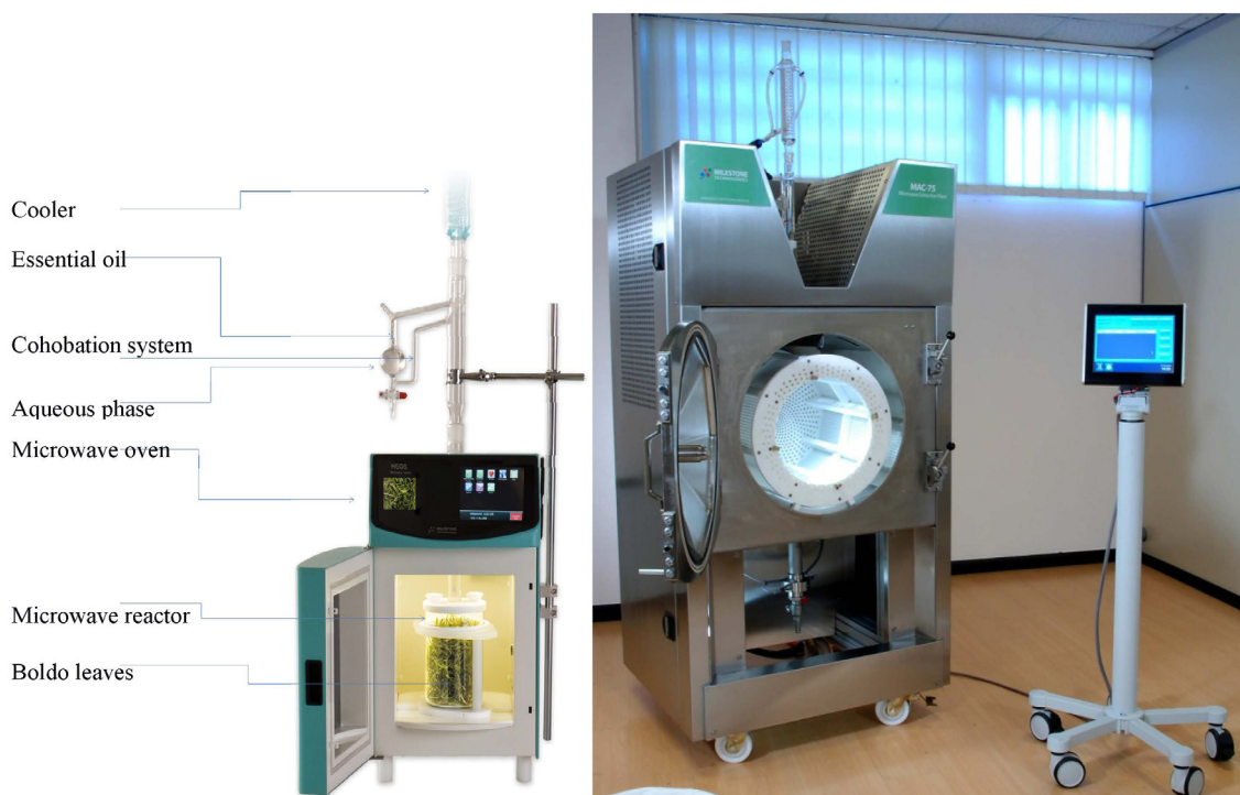
Figure 7. Laboratory and pilot scale microwave extractor.
