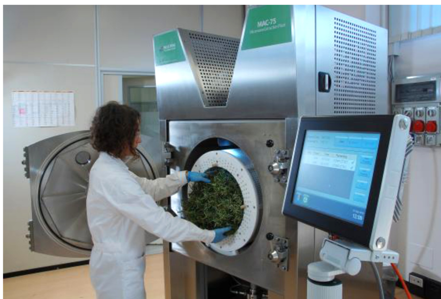
Fig. 1. Solvent free microwave extraction: from laboratory to pilot scale.
