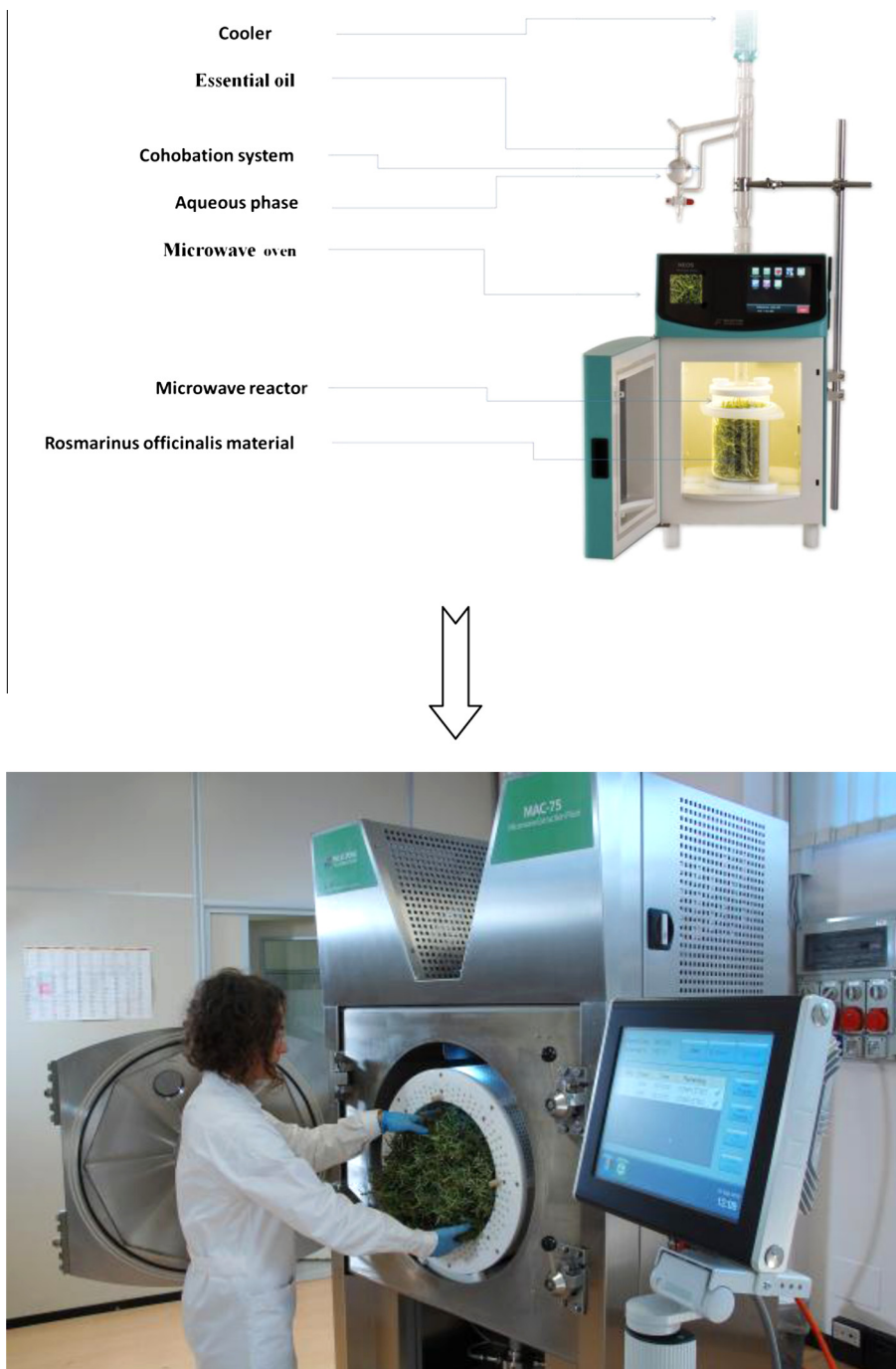
Fig. 1. Solvent free microwave extraction: from laboratory to pilot scale.
