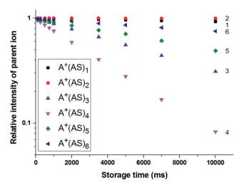
Fig. 4 Relative intensity of the parent ions  $A^+(AS)_n$  (with n=1-6) for different ion-trap storage times. Cluster size n is also indicated next to the data series for clarity. Note the semi-logarithmic scale.
