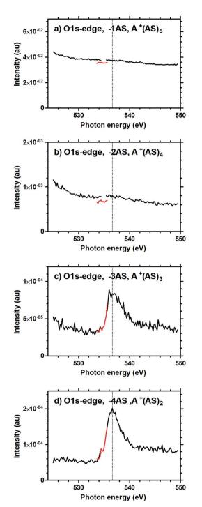
Fig. 1 Relative intensity of fragmentation peaks corresponding to the loss of 1 AS unit (panel a), 2 AS units (panel b), 3 AS units (panel c) and 4 AS units (panel d) from the  $A^+(AS)_6$  cluster ion in the energy region of the oxygen-1s absorption edge. Original measurement in black (data points lost for 534.2–535.4 eV); completing measurement in red. The vertical dotted line is included to guide the eye.
