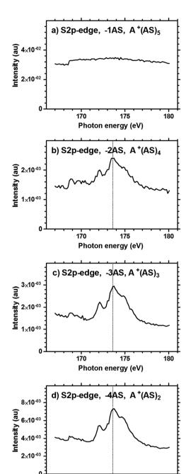
Fig. 3 Relative intensity of fragmentation peaks corresponding to the loss 1 AS unit (panel a), 2 AS units (panel b), 3 AS units (panel c) and 4 AS units (panel d) from the  $A^+(AS)_6$  cluster ion in the energy region of the sulphur-2p absorption edge. The vertical dotted line is included to guide the eye.
