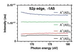
Fig. 5 Relative intensity of the fragmentation peaks corresponding to loss of a single AS unit loss from the clusters  $A^+(AS)_6$ ,  $A^+(AS)_5$ , and  $A^+(AS)_5$  in the energy region of the S2p absorption edge.
