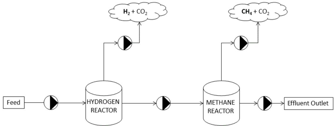
**Figure 2. Integrated hydrogen and methane production in a two-stage system.**
