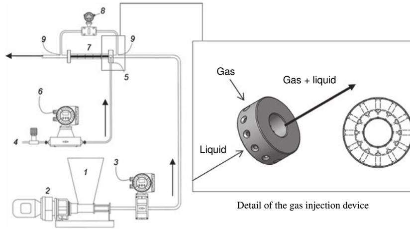
**Fig. 1.** Experimental rig (1) liquid feed; (2) pump; (3) volumetric liquid flow meter; (4) gas supply; (5) absolute gas pressure sensor, (6) mass gas flow meter; (7) static mixer; (8) differential pressure sensor; (9) temperature sensors. The gas injection device is zoomed on the right of the figure.
