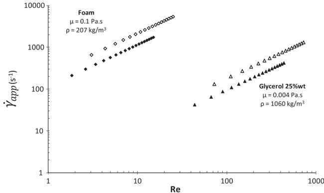
**Fig. 5.** Evolution of apparent shear rates in SMX+6 (hollow symbols) and SMX10 (full symbols) respectively with flow of foam ( $\diamond$ ,  $\alpha = 0.8$  and  $\mu = 0.1$  Pa.s) and flow of a glycerol solution ( $\blacktriangle$ ) versus Reynolds numbers.
