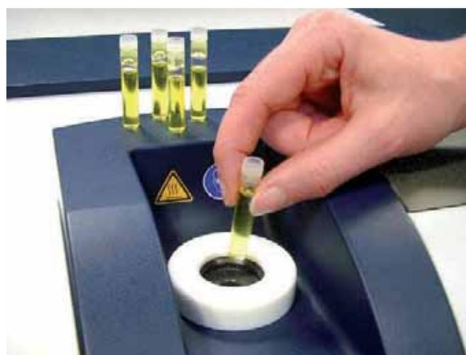
**Figure 1:** Measurement of frying oils with FT-NIR spectroscopy
