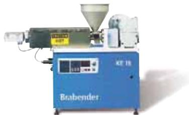
The Extruder KETSE 20/40D is designed for more complex extrusion tasks
