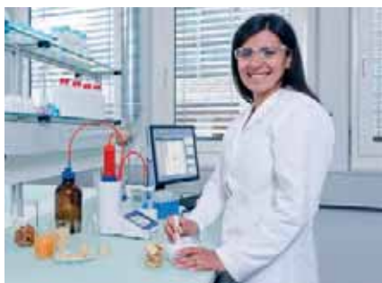
A lab technician is preparing a snack food sample for the sodium analyser by shredding with piston and mortar
