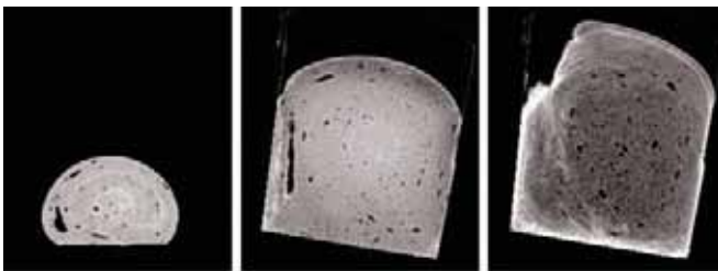
Figure 1: X-ray image of bread dough during proving and baking, showing dough at the start and end of proving and at the end of baking
