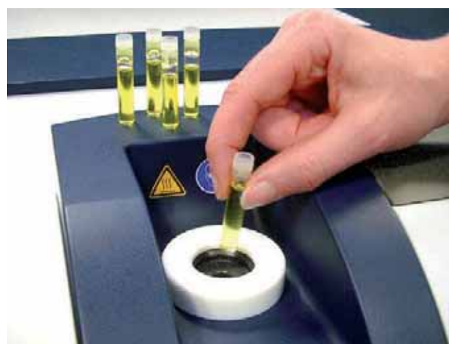
Figure 1: Measurement of frying oils with FT-NIR spectroscopy
