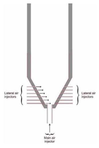
Figure 3: Sketch of the modified spouted bed with lateral air injections
