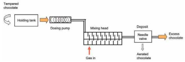
Figure 2: Flow diagram of a typical process used to incorporate gas into liquid chocolate (Taken from: Bubble-Included Chocolate: Relating Structure with Sensory Response J. Hadelt, S.T.Beckett, and K. Niranjan, Journal of Food Science, Vol. 72, Nr. 3 (2007) doi: 10.1111/j.1750-3841.2007.00313)
