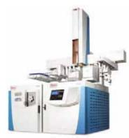
Figure 1: Thermo Scientific TSQ 8000 Triple Stage Quadrupole Mass Spectrometer
