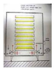
**Figure 5:** Cross-section of short good drying diagram. Courtesy of Braibanti
