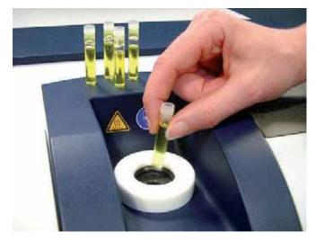
Figure 1: Measurement of frying oils with FT-NIR spectroscopy
