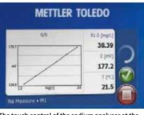
The touch control of the sodium analyser at the end of a multiple standard addition, showing the linearity of the test as well as the result
