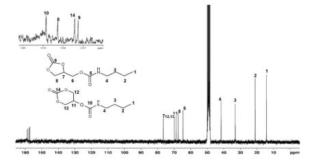
**Figure 2.**  $^{13}$ C NMR spectrum of (2-oxo-1,3-dioxolan-4-yl)methyl butylcarbamate (N°4A) and 2-oxo-1,3-dioxan-5-yl butylcarbamate (N°5A) in CD<sub>3</sub>OD.
