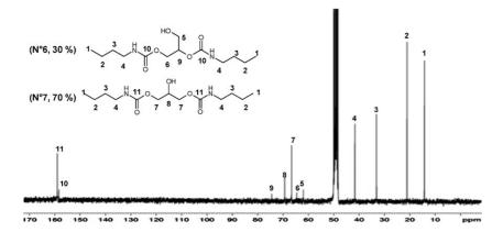
**Figure 3.**  $^{13}$ C NMR spectrum of 3-hydroxypropyl-1,2-di(butylcarbamate) (N°**6**A) and 2-hydroxypropyl-1,3-di(butylcarbamate) (N°**7**A) in CD<sub>3</sub>OD.
