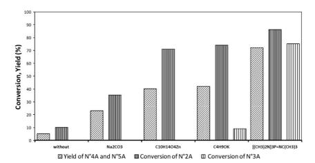
**Figure 4.** Influence of the catalyst on the transesterification of  $\alpha$  and  $\beta$  *N*-butylHU (N°2A and N°3A) with DMC (DMC/HU = 2, 7 h, 80°C); conversions (%) of  $\alpha/\beta$  *N*-butylHU and yield (%) of 5CGC (N°4A) and 6CGC (N°5A) calculated by Zgig <sup>13</sup>C NMR.
