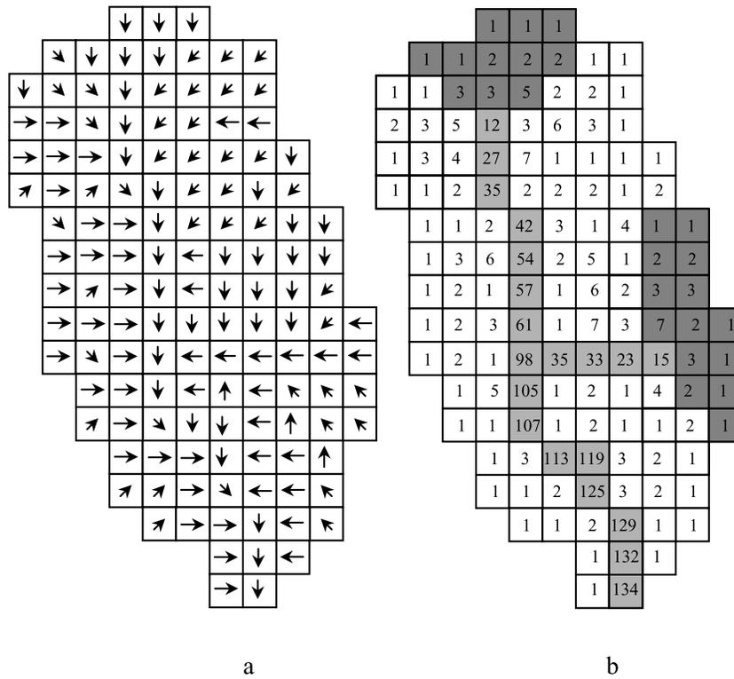
**Figure 2.** (a) Identification of the drainage direction of each pixel from a digital elevation model (DEM). (b) Contributing drainage area (number of pixels) at each pixel of the catchment. The channel network extracted with an upstream cutoff area  $A = 10$  pixels is shown in lighter gray, and the corresponding upstream subcatchments is in darker gray.
