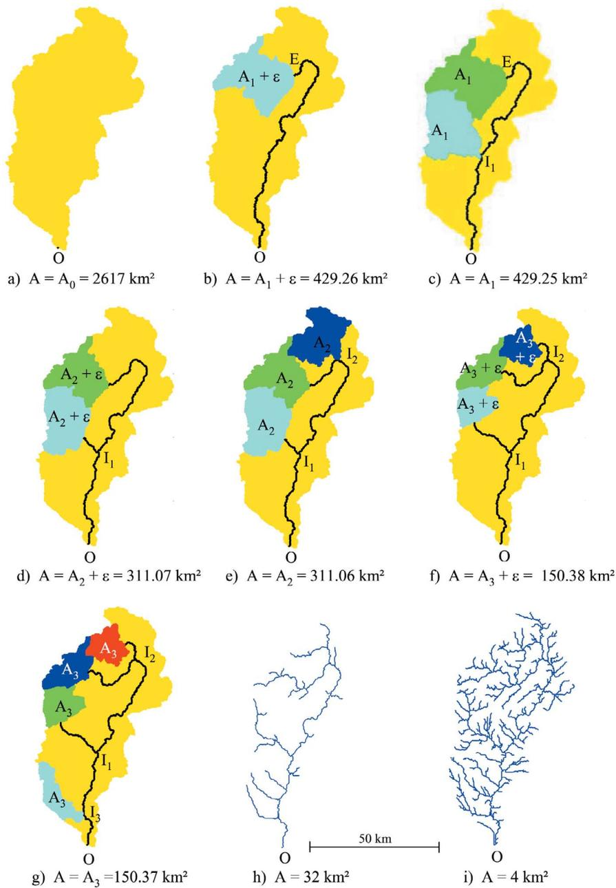
**Figure 3.** Example of the channel network of the Hérault catchment extracted for various values of the cutoff area  $A$ .
