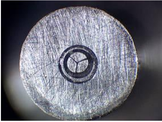
Fig. 2. Top view of three-segment probe with a diameter of 0.5 mm embedded in a tube with 3 mm outside diameter.
