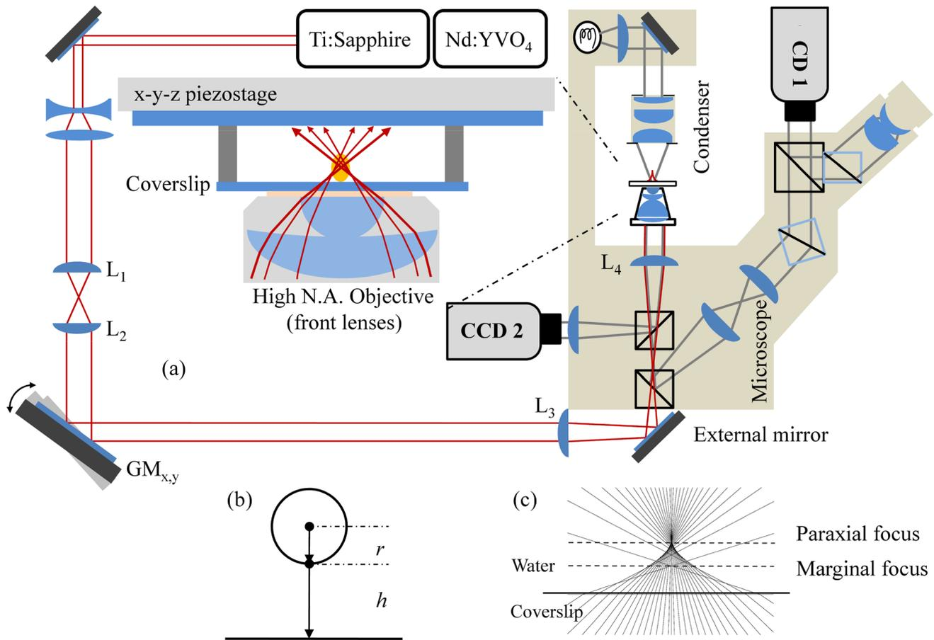
FIG. 1. (a) Simplified schematic layout of the optical tweezers system. (b) Sketch showing the trapped bead (radius  $r$ ) with respect to the surface at height  $h$ . (c) Ray-tracing representation of the refracted trapping beam, showing a shift between the marginal rays and the paraxial rays, which is responsible for an elongated focal volume (spherical aberration).
