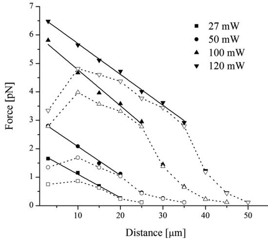
FIG. 2. Variation of the apparent drag force as a function of the distance to the wall, as deduced from measurements performed after calibrating the trap force at a distance of  $20 \mu\text{m}$  from the wall, with (solid lines, closed symbols) or without (dashed lines, open symbols) correction for the hydrodynamic wall effect, at different laser powers in the sample.
