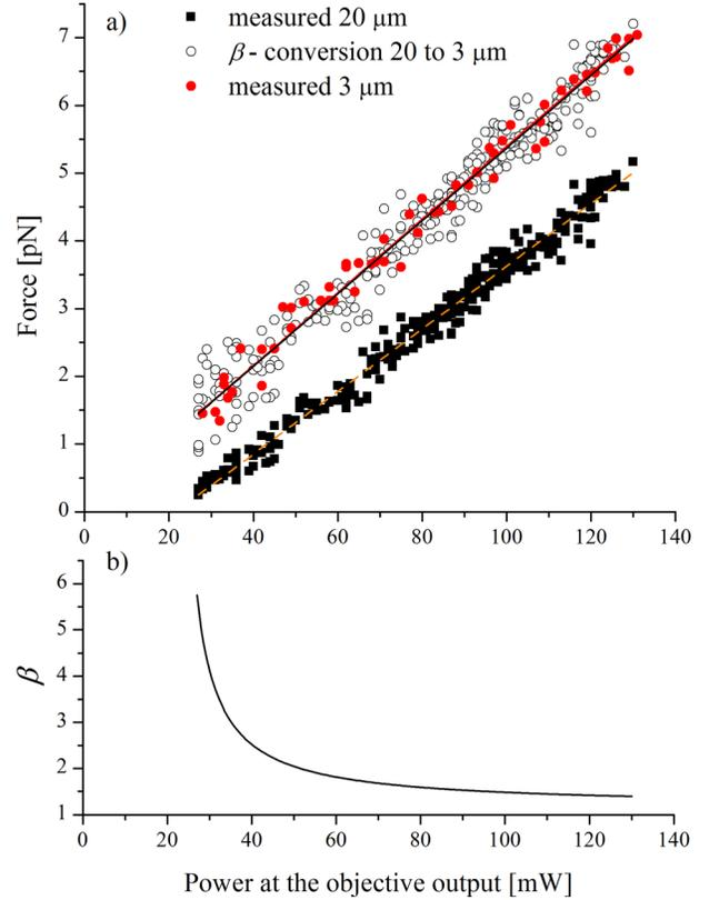
FIG. 4. (a) Wall-corrected drag force (pN) vs. laser power at the objective, measured at a distance of  $3\ \mu\text{m}$  (red closed circles) and  $20\ \mu\text{m}$  (black closed squares) from the surface. Experimental data taken at  $20\ \mu\text{m}$  and converted to the distance of  $3\ \mu\text{m}$  (open circles) though multiplication by  $\beta$ . (b) Conversion factor  $\beta$  described by Eq. (13).
