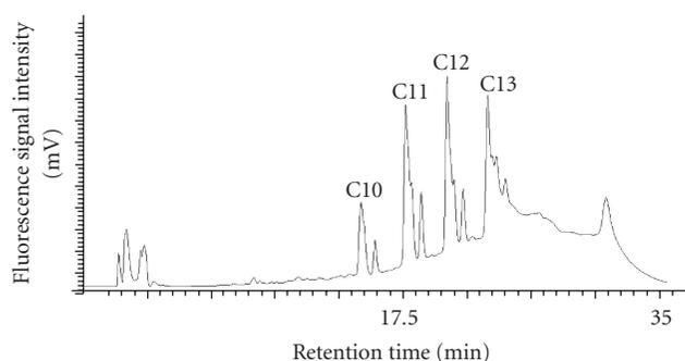
FIGURE 3: HPLC-FLD chromatogram obtained for carrot sample spiked with LASs ( $50 \mu\text{g g}^{-1}$  dry matter). Chromatographic condition: Inertsil ODS3 column of  $250 \times 4.6$  mm ( $5 \mu\text{g}$ ), flow rate =  $1.5 \text{ mL min}^{-1}$ , fluorescence detection (ex:  $225 \text{ nm}$ —em:  $305 \text{ nm}$ ),  $20 \mu\text{L}$  of injection volume.
