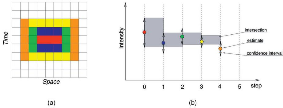
Fig. 2. (a) Spatio-temporal neighborhood: Colors correspond to iterations plotted in (b). (b) Confidence intervals: Circles represent estimates  $\hat{u}_{i,n}$  obtained at each iteration  $n$ . The gray rectangles represent the intersection between the current confidence interval and the previous one. As long as the estimate belongs to this intersection, the estimation process is updated.
