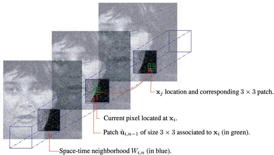
Fig. 1. Patch-based space-time framework. To each point of the image sequence is associated an estimated space-time neighborhood  $W_{i,n}$ . To each point  $x_j$  of this neighborhood is associated a  $3 \times 3$  patch ( $7 \times 7$  image patches are used in practice). Every weight  $\omega_{ij}$  is defined as a function of the distance between the patch centered in point  $x_i$  and the patch centered in point  $x_j \in W_{i,n}$ .
