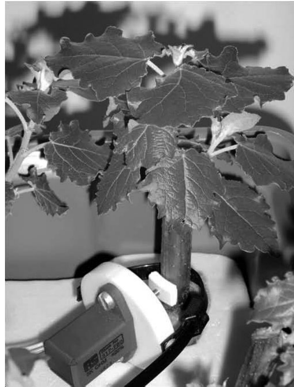
Fig. 1. Radial growth measured with a linear motion sensor on the stem of Populus tremula × Populus alba clone 717-1B4 cultivated under hydroponic conditions.
