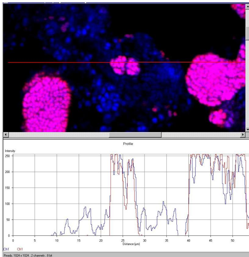
**Figure 1.** Determination of the threshold values for surface area measurement of the bacterial populations. Top. Zoom in of a digitized image of a nitrifying activated sludge sample simultaneously hybridized with the Cy3-labeled NEU23a probe specific of the *Nitrosomonas* group (in red) and the Cy5-labeled EUB338 general bacterial probe (in blue). Bottom. Grey level profile obtained across the red lane drawn on the image.
