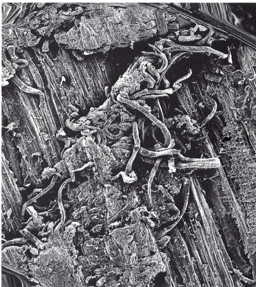
Fig 1: Scanning electron microscopy image of lignin fusion with cellulose fibers and wood cells (tracheids) immersed in it obtained during welding at 100 magnification showing the entangled and detached tracheids, a fused intercellular lignin mass and tracheids and fibers immersed in the fused lignin matrix.
