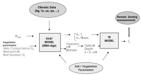
**Figure 4.** General principle of the coupling between ISBA-Ags and the TB model (approach II). The parameters to be retrieved from the  $T_B$  measurements were initial soil water content ( $R_{2\text{-INIT}}$ ) and the vegetation parameter (B/LAI).
