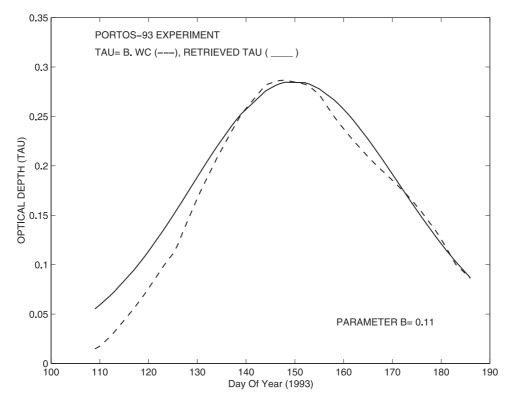
**Figure 6.** Comparison between retrieved (solid lines) and estimated (dashed lines) values of optical depth. Estimated values of optical depth ( $\tau_W$ ) were derived from ground measurements of the amount of water in the canopy  $W_C$  (kg/m<sup>2</sup>) according to  $\tau_W = b$ .  $W_C$ , where b = 0.11 (approach I).
