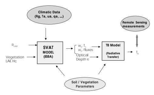
**Figure 3.** General principle of the coupling between Interactions between Soil-Biosphere-Atmosphere (ISBA) and the brightness temperature (TB) model (approach I). The variables to be retrieved from the  $T_B$  measurements were initial soil water content ( $R_{2\text{-INIT}}$ ) and time variations in optical depth  $\tau$ .
