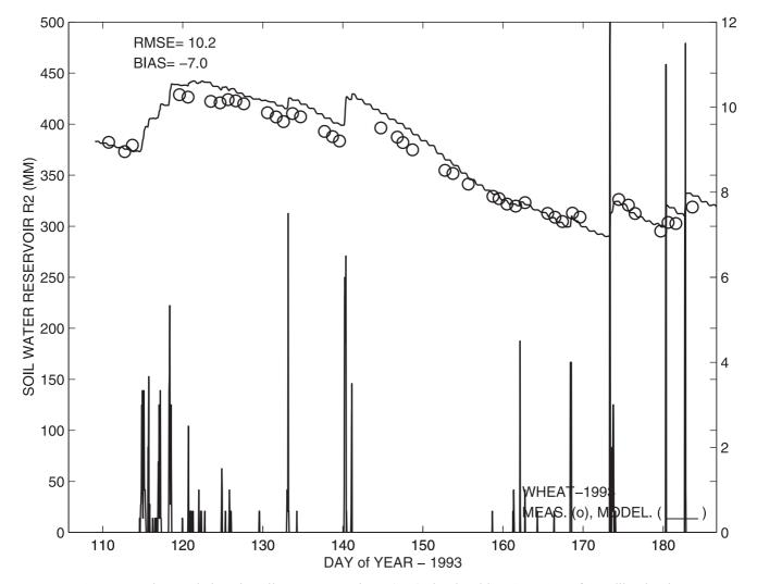
**Figure 7.** Time variations in soil water reservoir  $R_2$  (mm) simulated by ISBA-Ags after calibration by the assimilation process (approach II). The simulations (solid line) were compared with the observations (open circles). Rain and irrigation rates (mm h<sup>-1</sup>) are indicated by vertical solid lines.
