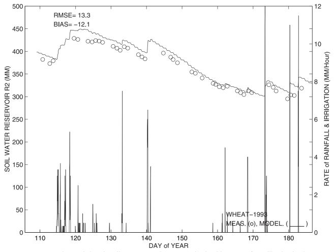
**Figure 5.** Time variations in soil water reservoir  $R_2$  (mm) simulated by ISBA after calibration by the assimilation process (approach I). The simulations (solid lines) were compared with the observations (open circles). Rain and irrigation rates (mm h<sup>-1</sup>) are indicated by vertical solid lines.
