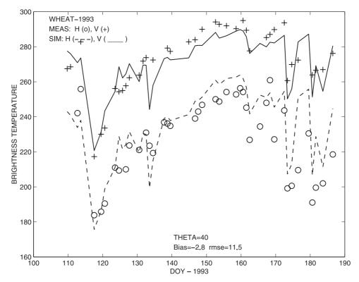
**Figure 9.** Comparison between measurements and simulations of brightness temperature  $T_B$  at  $\theta = 40^{\circ}$  at both H and V polarizations by the coupled ISBA-Ags/TB model (approach II, using b' = 0.07).
