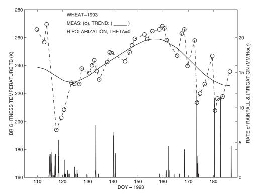
Figure 1. Microwave observations over the wheat field at view angle  $\theta = 0^{\circ}$ , at H polarization (open circles). The trend (solid lines) was obtained using a standard sliding window filtering technique. Rain and irrigation rates (mm h<sup>-1</sup>) are indicated by vertical solid lines.
