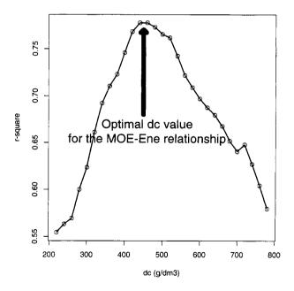
**Figure 6.** The selection of the optimal moving density criterion (dc) value for a given density parameter (here, energy [Ene]). The line shows the evolution of the strength of the relationship between the modulus of elasticity (MOE) and the parameter when the dc threshold varies from 200 to 800 g·dm<sup>-3</sup>. The optimal dc value coincides with the maximum  $r^2$ .
