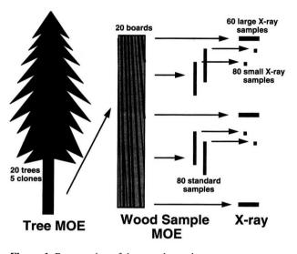
Figure 1. Presentation of the samples and measurements.
