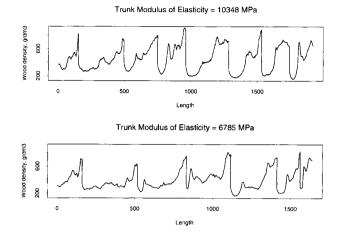
**Figure 3.** Upper panel: density profile of a stiff tree. Lower panel: density profile of a flexible tree. It is clear that the amount of 'high density wood' is larger in the stiff than in the flexible profile.
