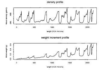
**Figure 2.** Upper panel: a raw density profile. Lower panel: a weighted density profile. The weight is proportional to the volume of the wood sheath correspondent to the local density profile value. We assume that the stem shape is cylindrical.
