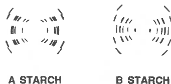
Figure 1. Schematic fiber diffraction pattern with vertical fiber axis of A- and B-starch.
