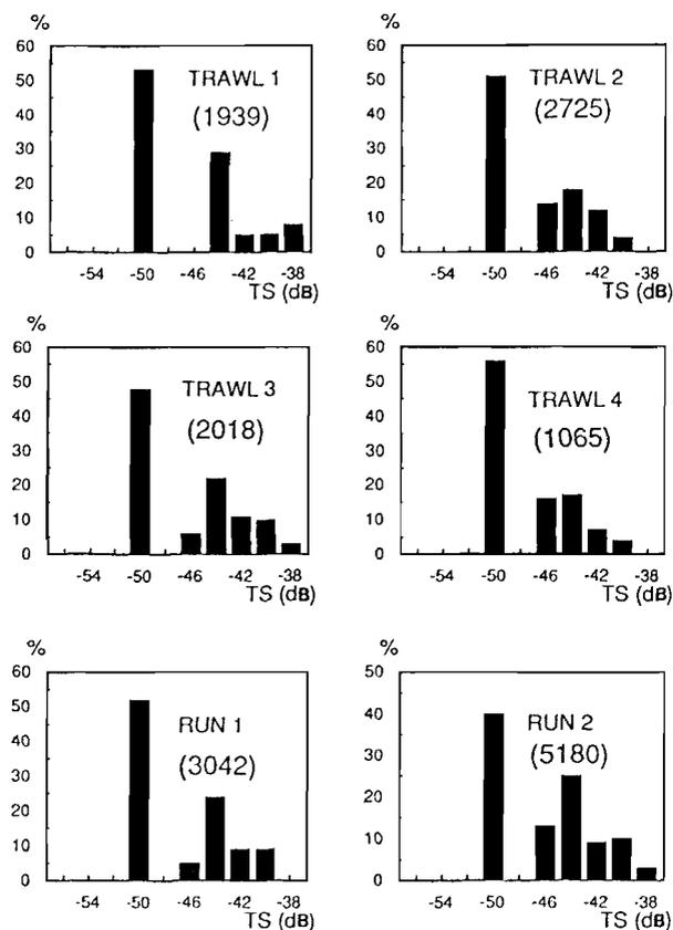
**Figure 4.** – Distribution of target strength estimated by HADAS (Hydro Acoustic Data Analysis System), expressed in units of target strength (log scale) for the four trawl hauls and the two runs, with indication of the number of single fish echoes in brackets.
