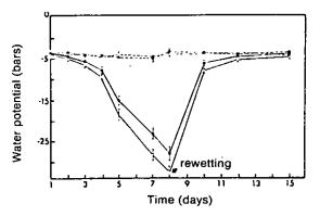
*Figure 1* Development of water potential in white clover plants under stress (---) and non-stressed (---) at 2 levels of potassium supply ( $K_0$ : O and  $K_1$ : •);  $K_1$  equivalent to 300 kg/ha  $K_2O$ .
