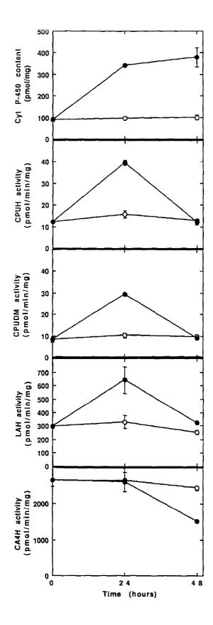
F1G. 3. Activities of chlorotoluron ring-methyl hydroxylase (0) and N-demethylase (e) in presence of diclofop in microsomes isolated from wheat cells that had been pretreated with 300  $\mu$ ,M 2,4-D for48 hr. Control values **•**) were obtained during incubations without microsomal proteins or without cofactor.
