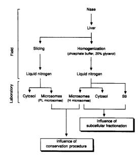
Fig. 1. Protocol for liver preparation and subcellular fractionation.
