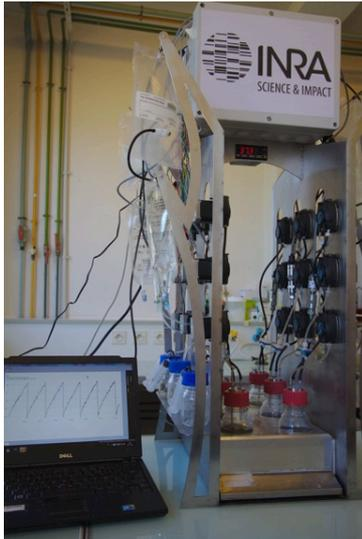
Figure 1: Module of six chemostats with the computer that controls the pumps and collects the data.
