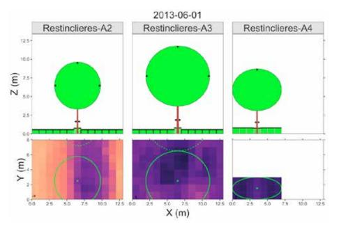
A snapshot of one day of three Hi-sAFe simulations. The top row illustrates a horizontal projection of the modelled scene. The bottom row shows a top-down view of the scene, with cell color proportional to shade by the tree on the crop (darker colors indicate more shade).
