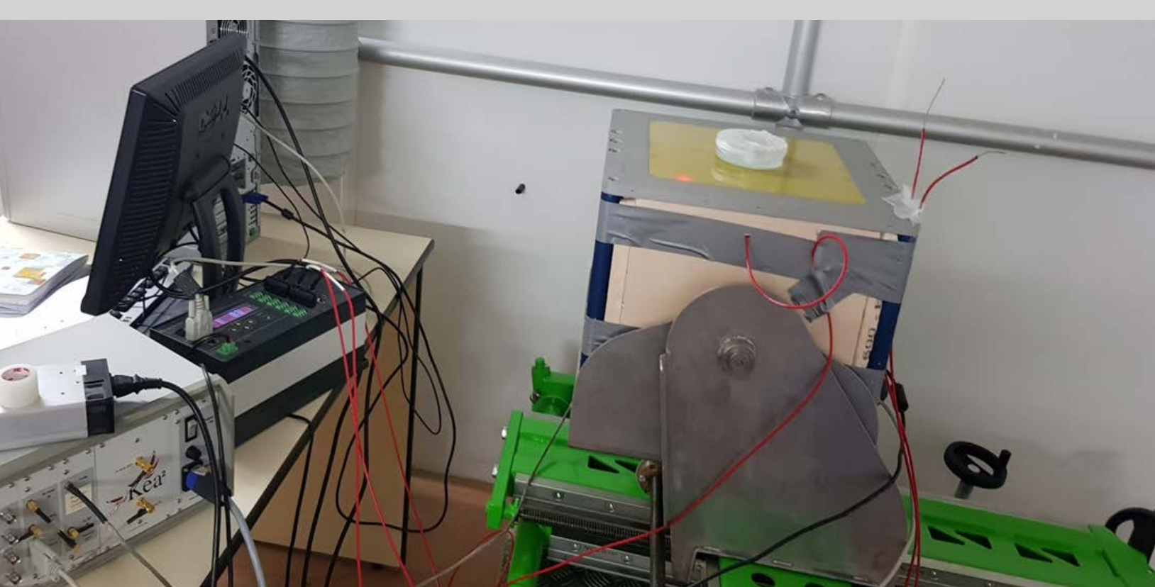
Figure 5 : identical experimental setup as in figure 1 except that the magnet is insulated with a 4-cm extruded polystyrene plate
